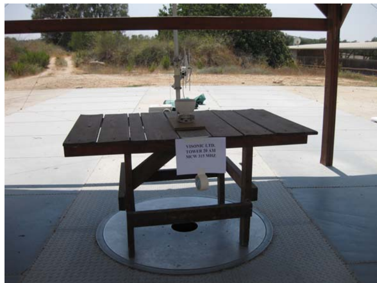
Figure 5. Open Site Radiated Emission Test
