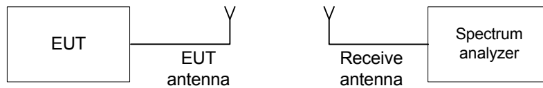
Figure 7.3.1 Hopping frequencies test setup
