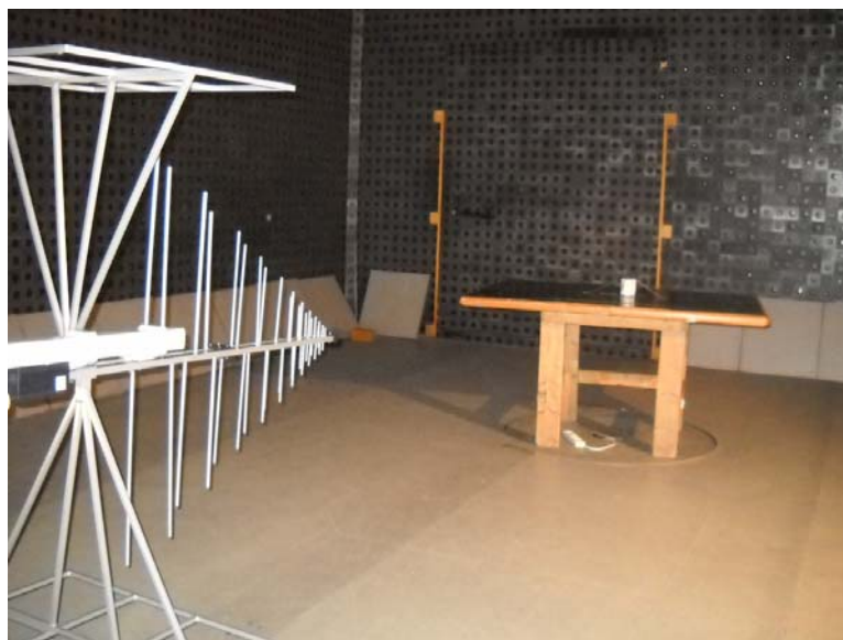
Photograph 8.1.1 Setup for radiated emission measurements
