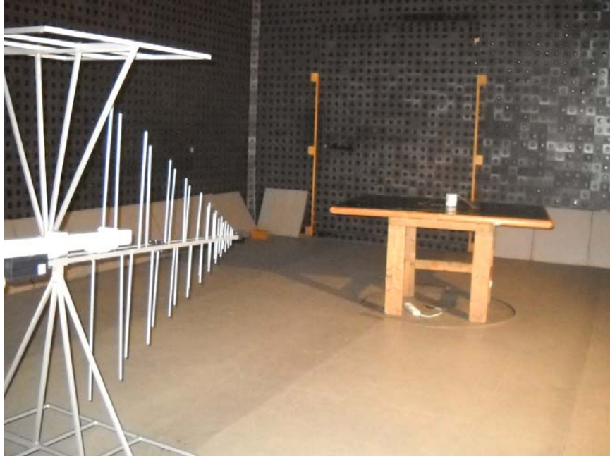
Photograph No.2 Setup for carrier field strength, OBW, spurious emission field strength measurements in the anechoic chamber in 30 – 1000 MHz range
