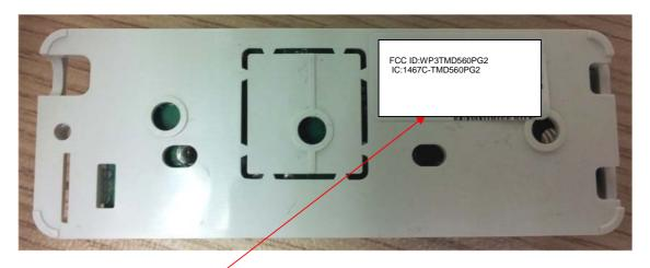
Label with **FCC ID:WP3TMD560PG2** and **IC:1467C-TMD560PG2** is located at the rear side panel. The statement according to FCC part 15 §15.19(a)(3) is placed in User's Guide, page 4 (Application exhibit User\_manual\_22354).
