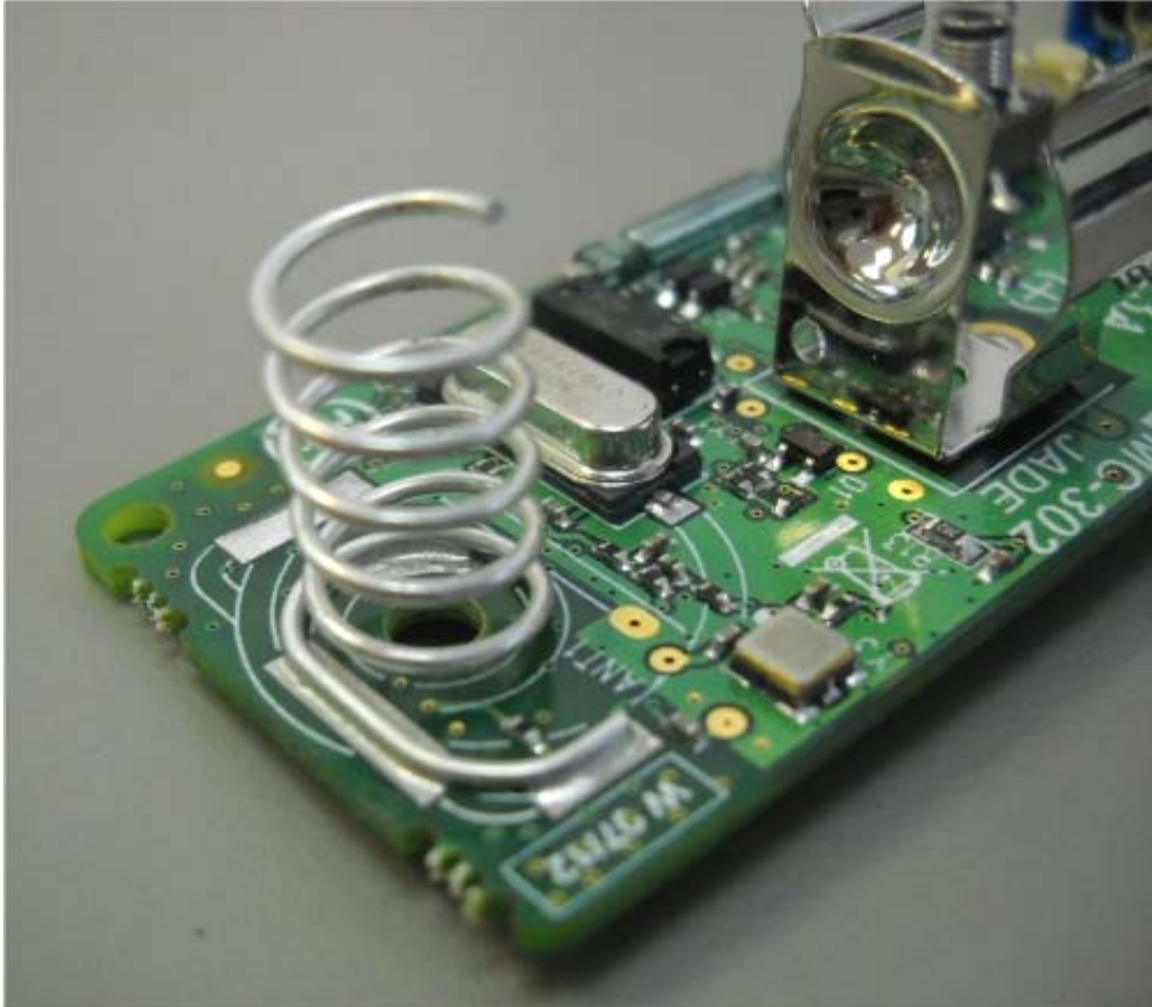
Photograph No.3 Temperature detector TMD-560 PG2 antenna
