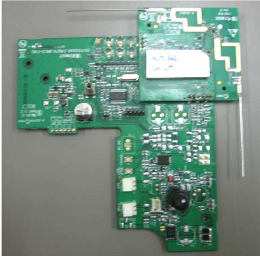
Photograph No.4 SR-730 PG2 wireless outdoor siren motherboard with FDD radio module
