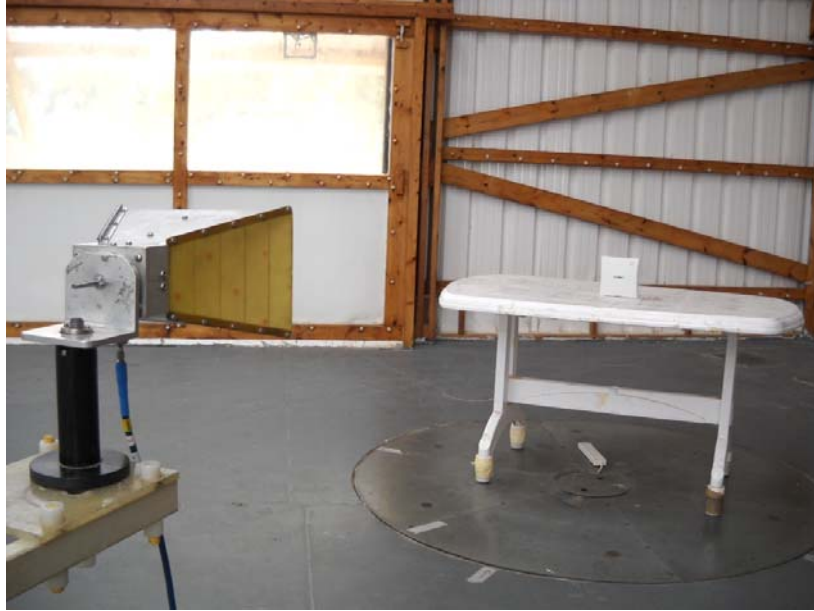
Photograph No.4 Setup for carrier and spurious emission field strength measurements at the OATS above 1000 MHz range
