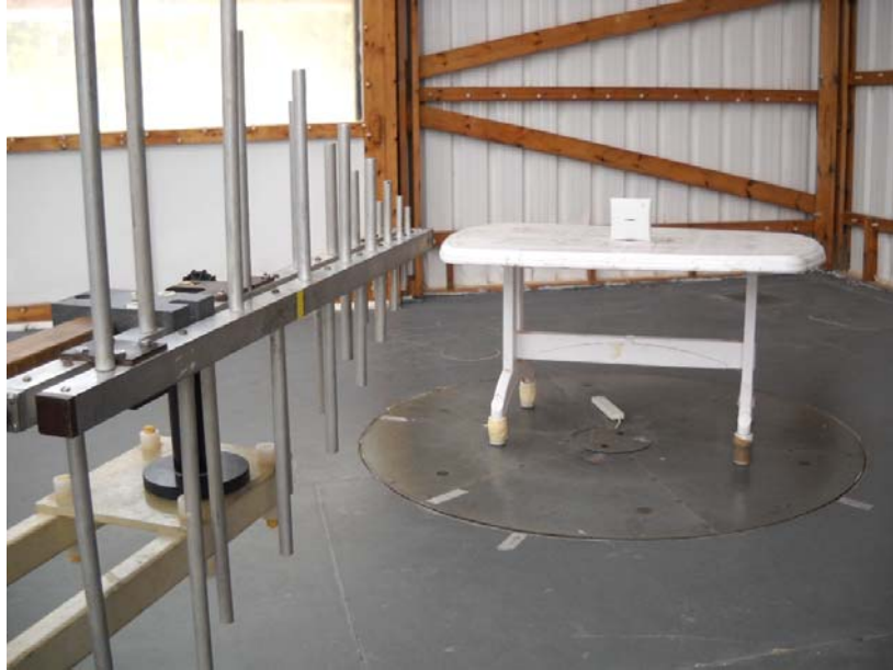
Photograph No.3 Setup for carrier, OBW, hopping frequencies and spurious emission field strength measurements at the OATS in 30 – 1000 MHz range
