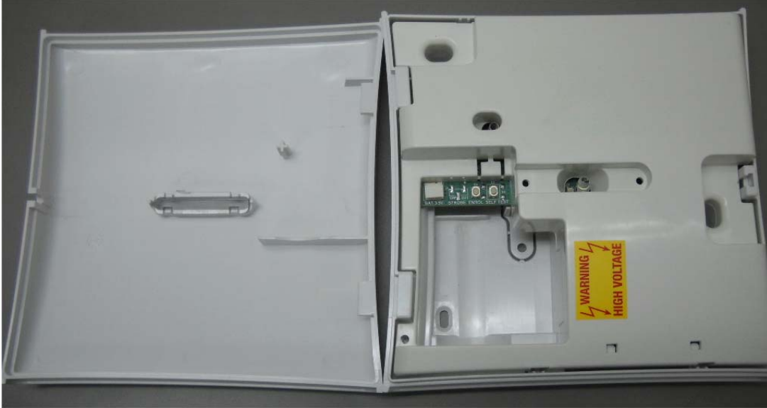
Photograph No.1 SR-720 PG2 wireless indoor siren internal view
