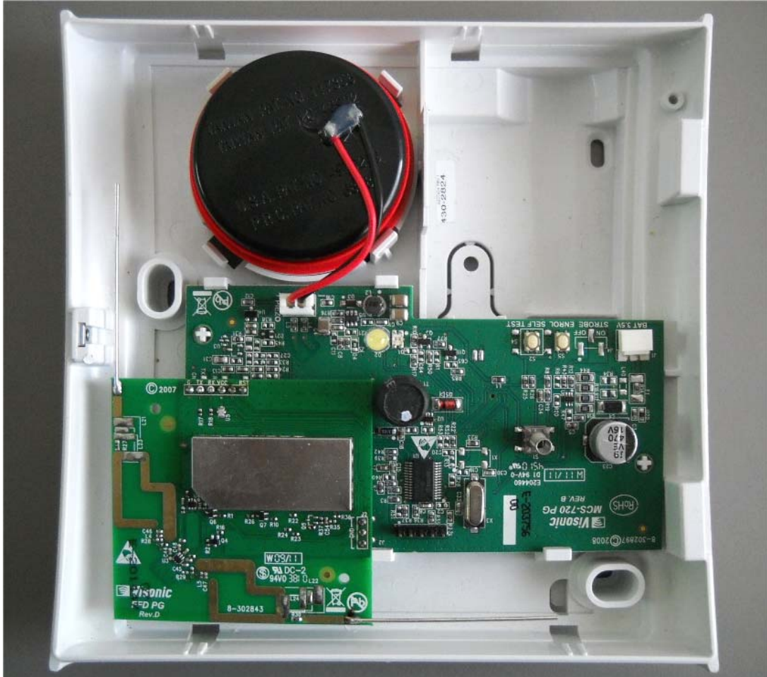
Photograph No.2 SR-720 PG2 wireless indoor siren internal view
