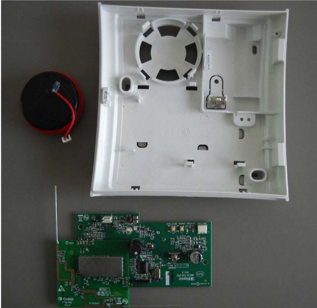
Photograph No.3 SR-720 PG2 wireless indoor siren with removed parts
