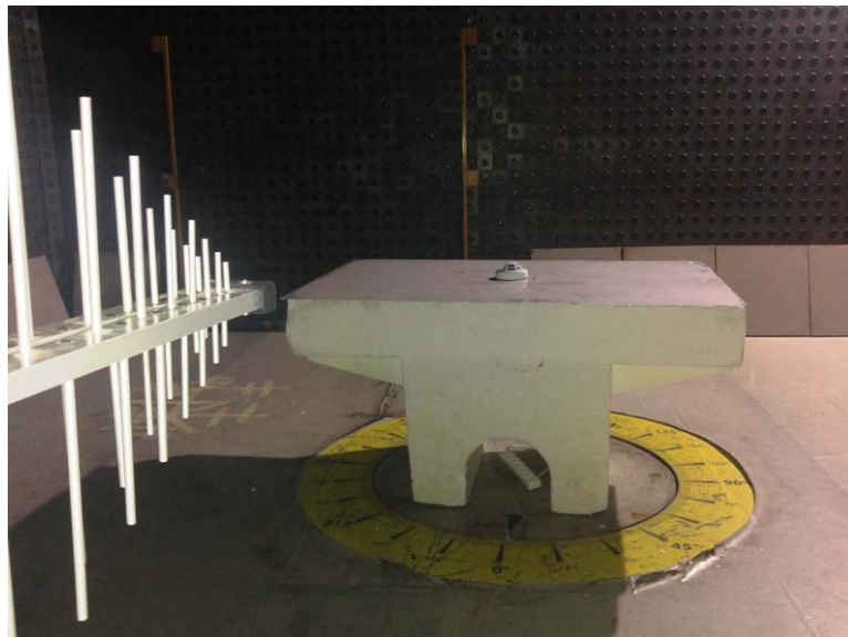
Photograph 8.1.1 Setup for radiated emission measurements
