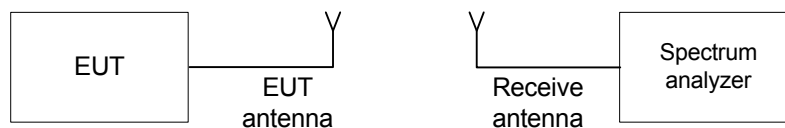
Figure 7.2.1 Carrier frequency separation test setup
