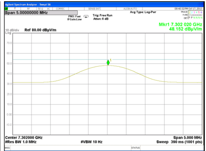
Plot 7.7.38 Radiated emission measurements at the eighth harmonic of mid carrier frequency
