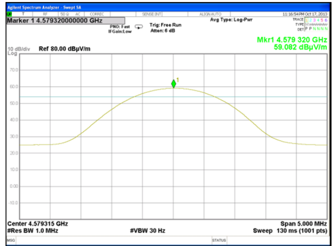
Plot 7.7.30 Radiated emission measurements at the fifth harmonic of high carrier frequency
