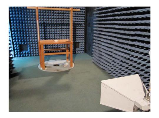
${\bf Photograph~No.4}\\ {\bf Setup~for~carrier~emission~field~strength~measurements~at~the~OATS~in~30-1000~MHz~range}$
