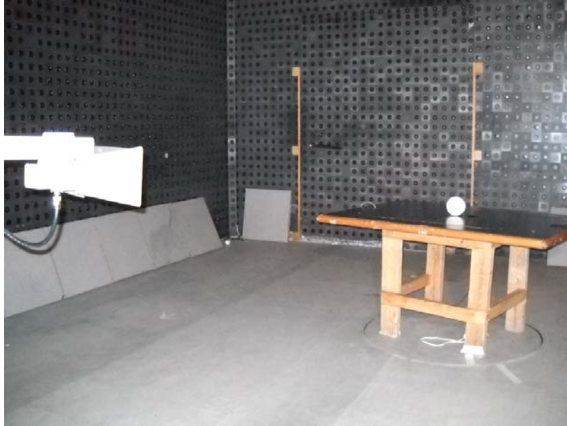
Photograph No.3 Setup for carrier and spurious emission field strength measurements in the anechoic chamber above 1000 MHz range
