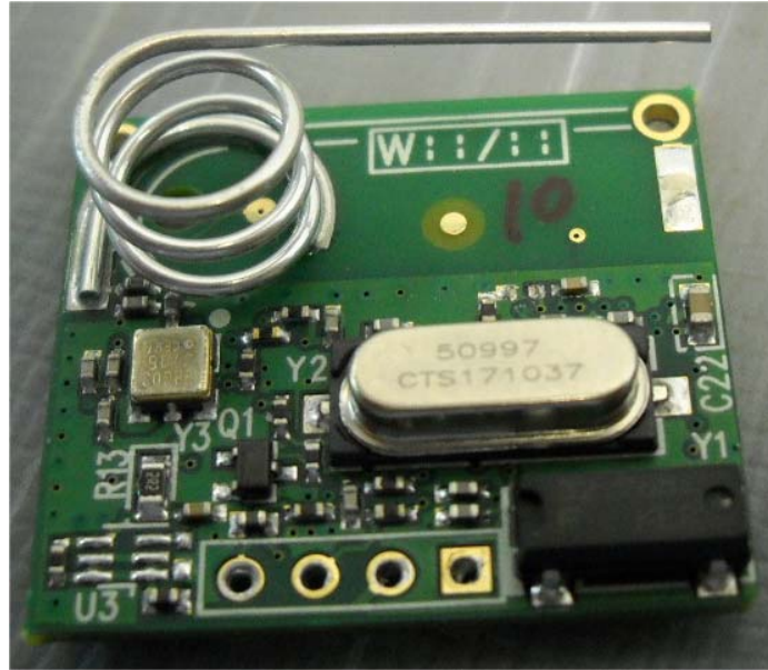
Photograph No.5 Detector RFD module front view
