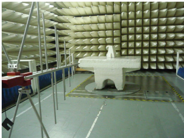
Photograph 8.1.1 Setup for radiated emission measurements, general view
