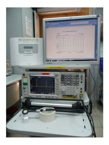
Photograph No.7 Setup for band edge emissions measurements
