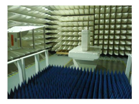
Photograph No.5 Setup for hopping parameters measurements
