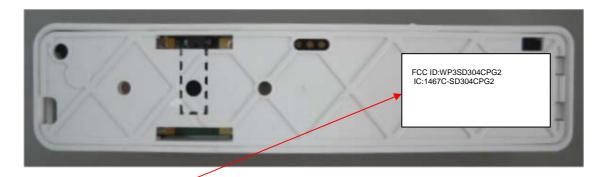
Label with FCC ID:WP3SD304CPG2 and IC:1467C-SD304CPG2 is located at the rear side panel of the shock detector. The statement according to FCC part 15 §15.19(a)(3) is placed in User's Guide, page 4 and page 5 (Application exhibit SD-304C\_UserMan).
