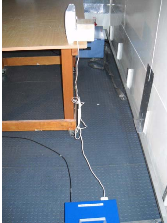
Photograph No.5 Setup for conducted emission measurements on AC power lines
