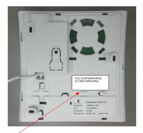
Label with FCC ID:WP3RP610PG2 and IC:1467C- P610PG2 will be located at the rear side panel.
