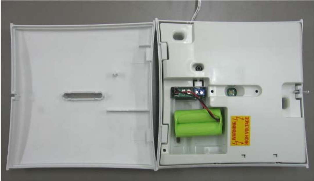
Photograph No.1 RP-610 PG2 wireless repeater internal view
