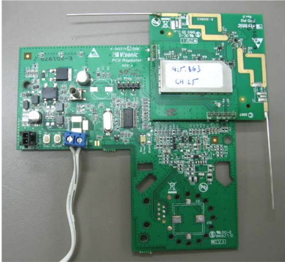
Photograph No.3 RP-610 PG2 wireless repeater motherboard with FDD radio module
