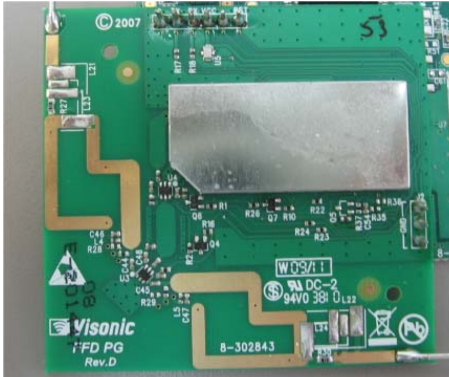
Photograph No.5 FFD RF module front view
