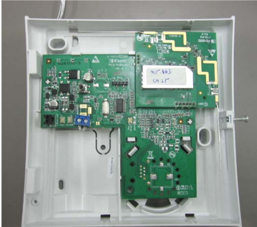
Photograph No.2 RP-610 PG2 wireless repeater internal view
