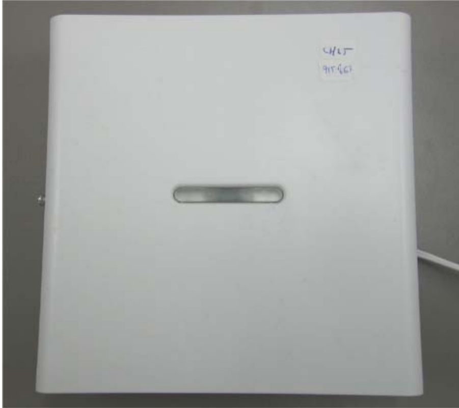
Photograph No.1 RP-610 PG2 wireless repeater front view
