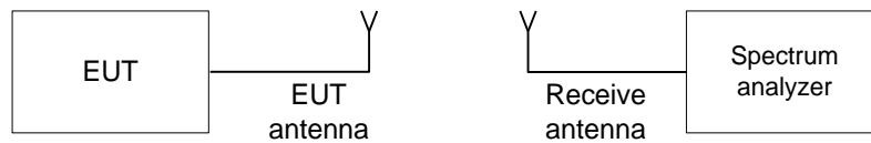
Figure 7.1.1 The 20 dB bandwidth test setup
