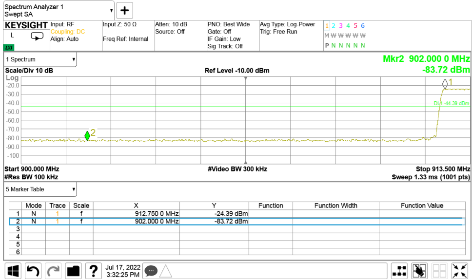
Plot 7.7.4 The highest band edge emission at high carrier frequency with hopping function enabled
