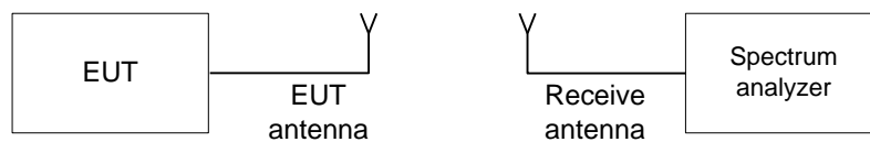
Figure 7.7.1 Band edge emission test setup
