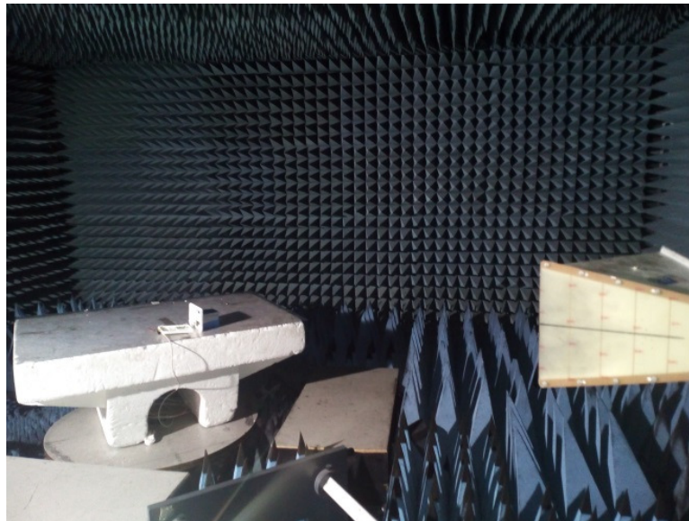
Photograph 8.1.3 Setup for radiated emission measurements, EUT cabling
