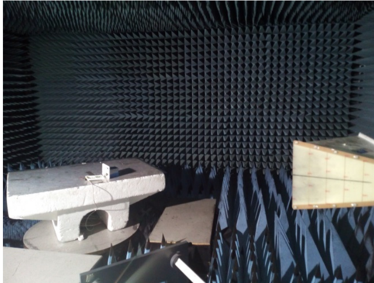
Photograph 8.1.2 Setup for radiated emission measurements
