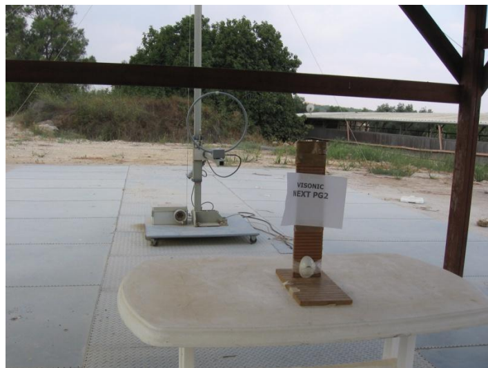
Figure 6. Radiated Emission Test
