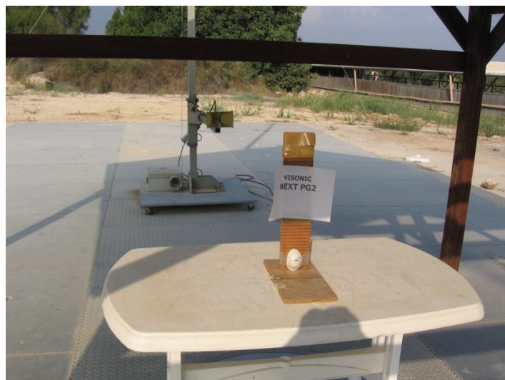
Figure 8. Radiated Emission Test
