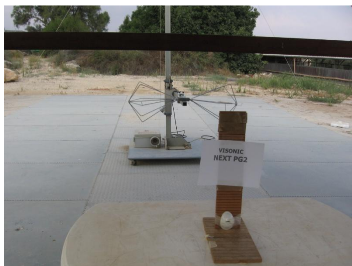
Figure 7. Radiated Emission Test
