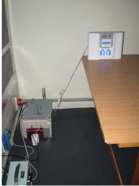
Photograph No.8 Setup for conducted emission measurements on AC power lines
