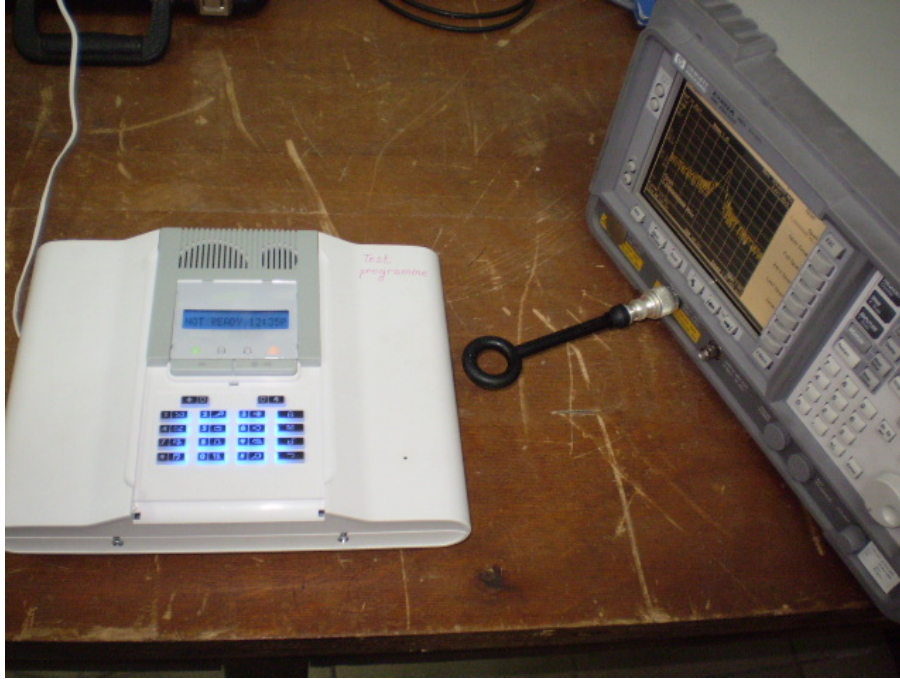
Photograph No.6 Setup for occupied bandwidth test
