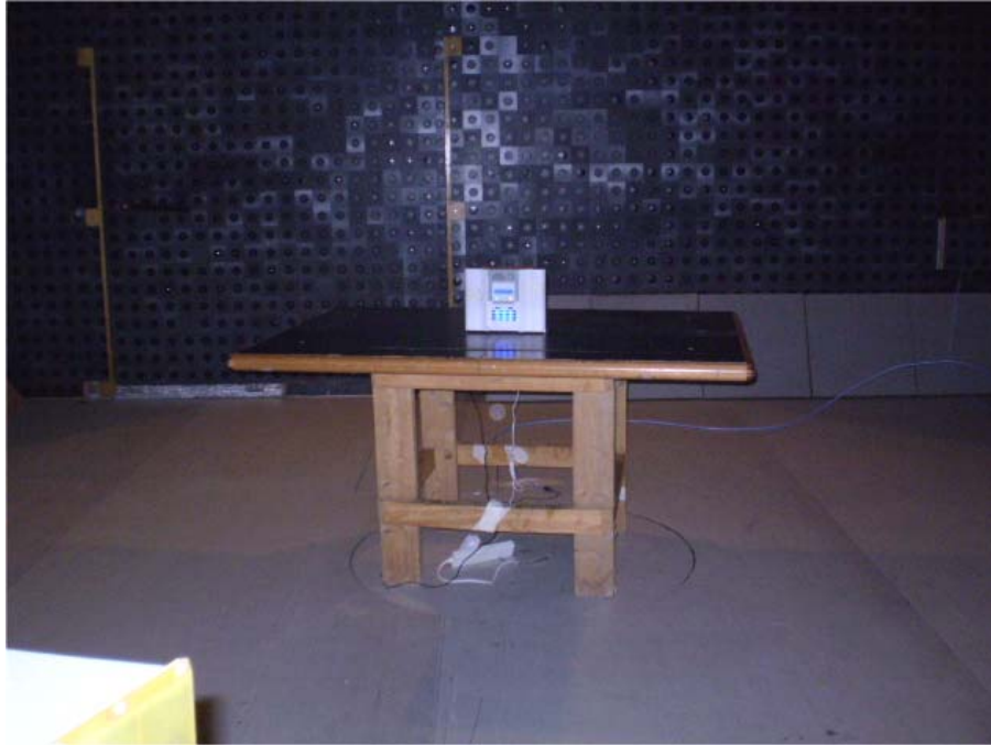
Photograph No.3 Setup for spurious emission field strength measurements in anechoic chamber above 1000 MHz
