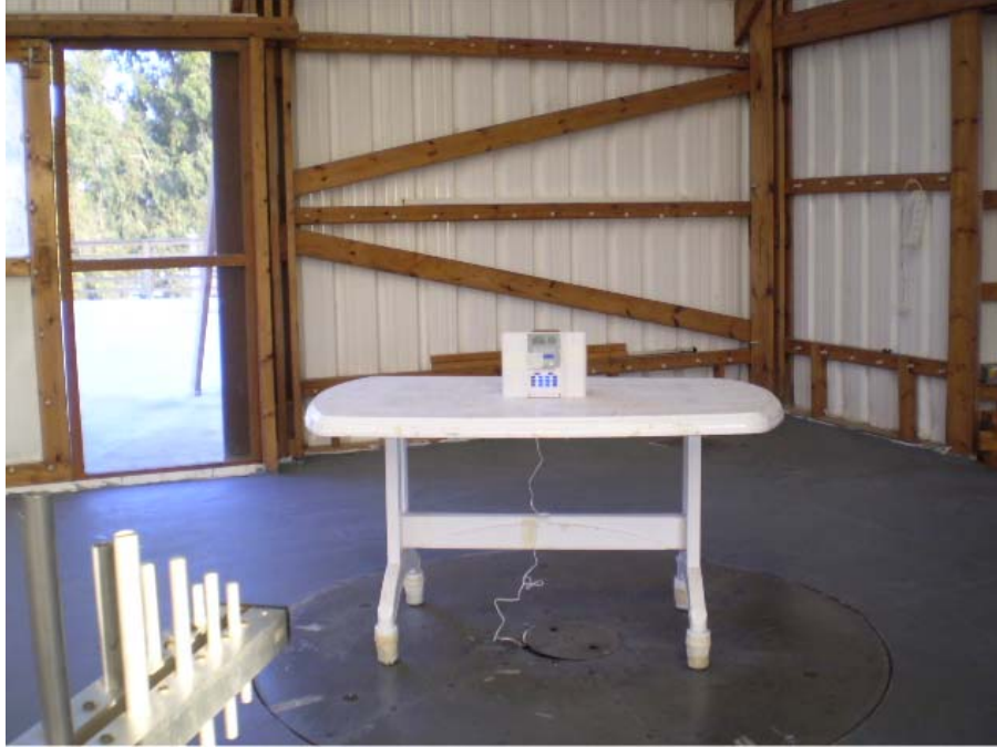
Photograph No.5 Setup for output power as per section 15.231 and spurious emission field strength measurements at OATS from 30 to 1000 MHz
