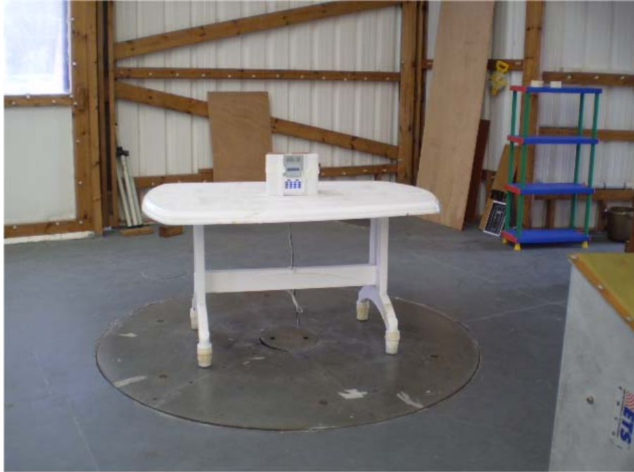
Photograph No.7 Setup for spurious emission field strength measurements at OATS above 1000 MHz
