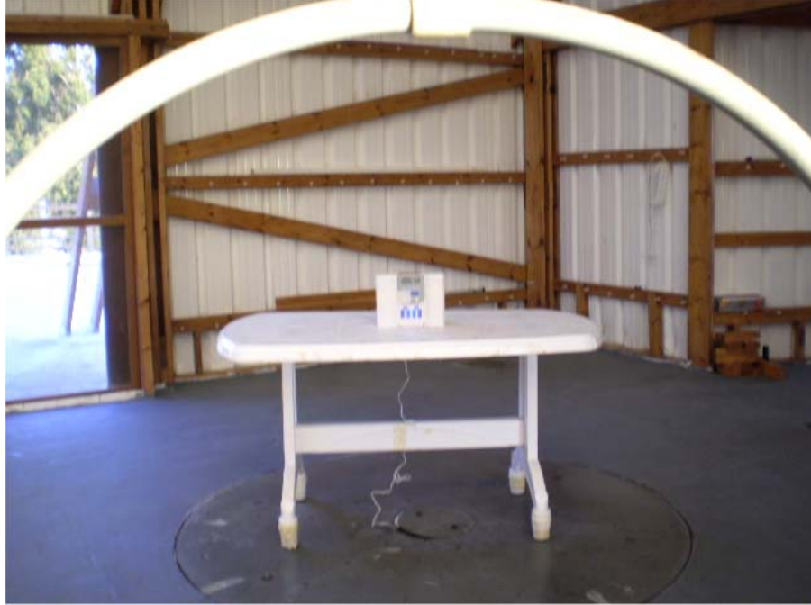
Photograph No.4 Setup for output power measurements as per section 15.209 at OATS
