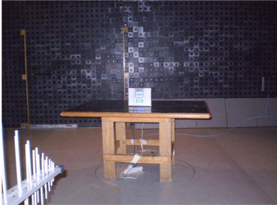
Photograph No.2 Setup for spurious emission field strength measurements in anechoic chamber from 30 to 1000 MHz
