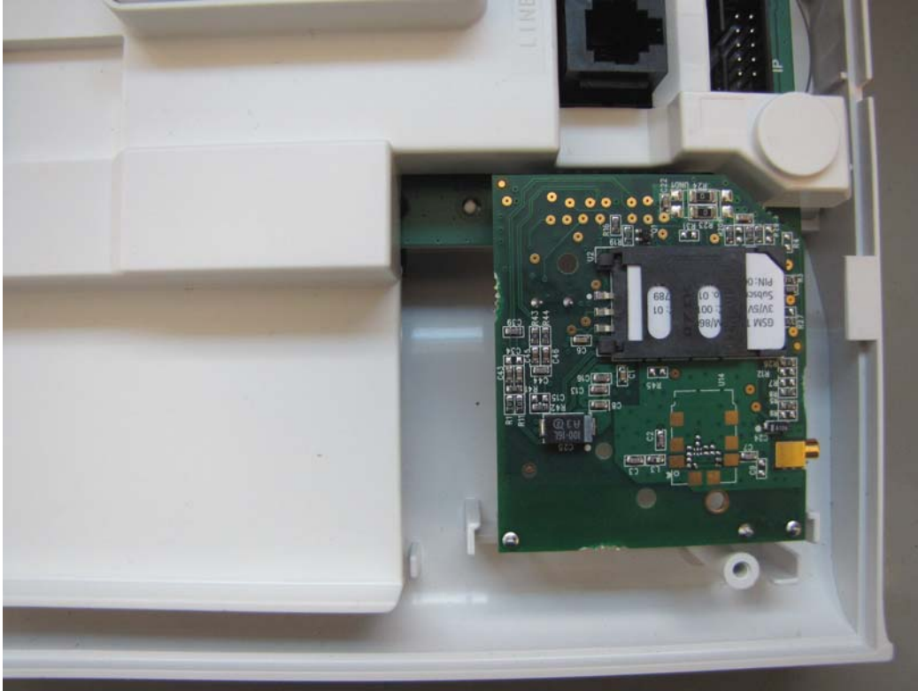
Photograph No.3 PowerMaxComplete GSM modem with cover removed view
