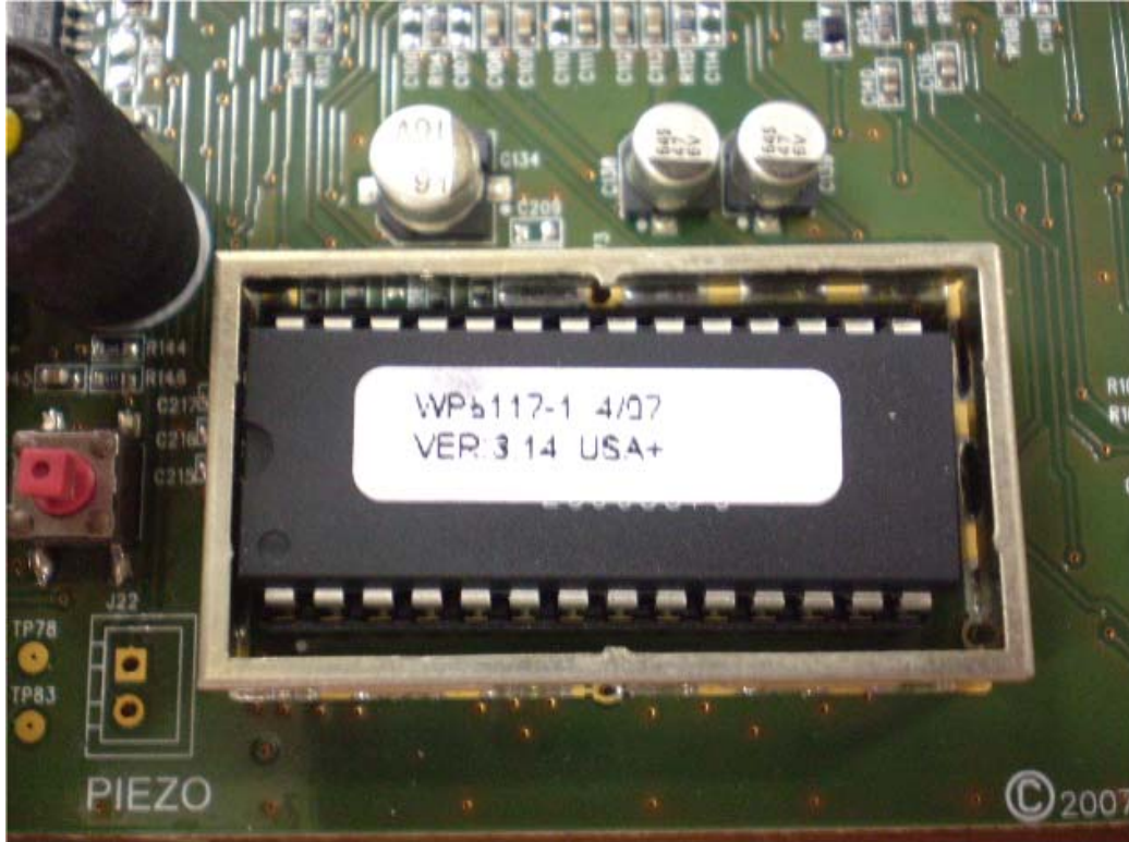
Photograph No.8 Main PCB front side view with shield removed
