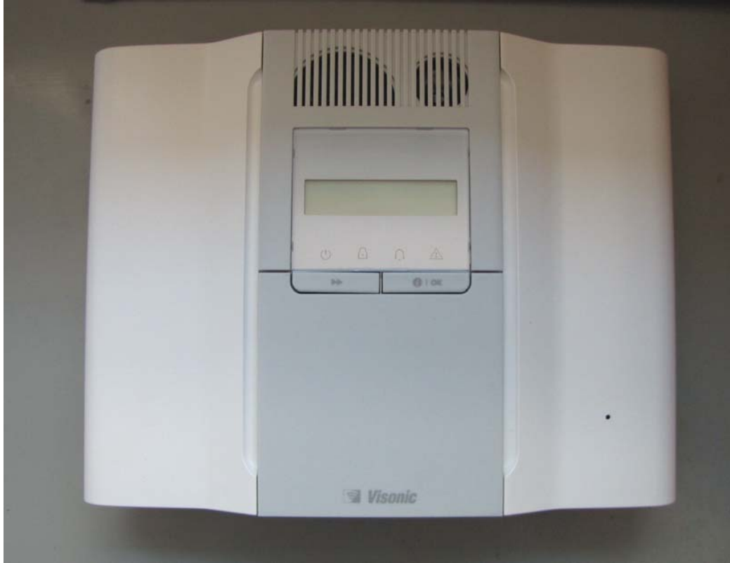
Photograph No.1 PowerMaxComplete control panel general view
