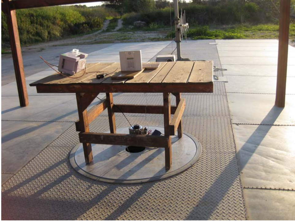
Figure 6. Inter-modulation Radiated Emission Test
