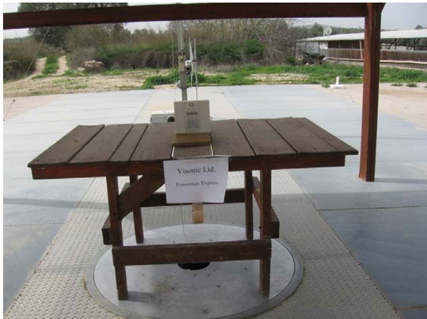
Figure 5. Radiated Emission Test
