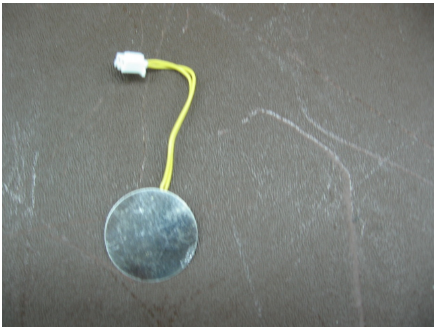
Figure 19: Siren (Inside Unit)
