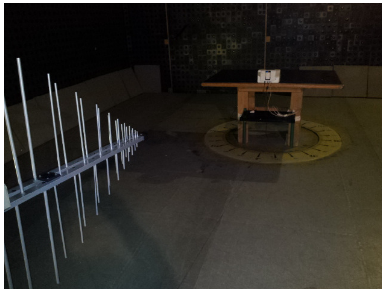
Photograph 8.2.2 Setup for radiated emission measurements, EUT cabling
