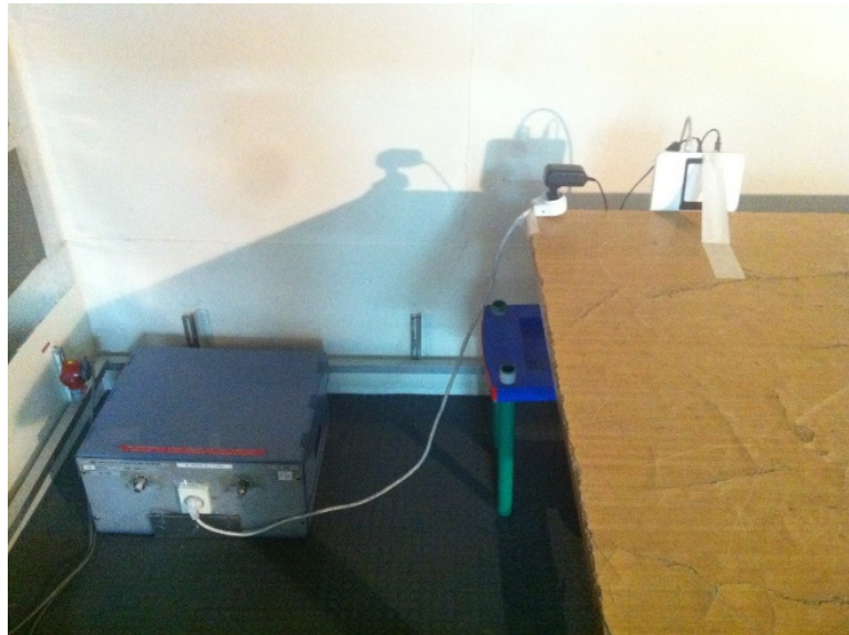
Photograph 8.1.1 Setup for conducted emission measurements
