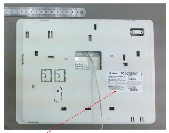
Label with FCC ID:WP3PMASTER20G2 and IC:1467C-PMASTER20G2 will be located at the rear side of the panel.
