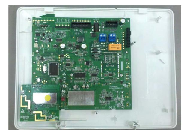
Photograph No.2 PMASTER-33 control panel internal view
