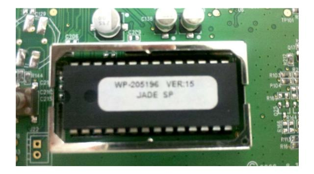
Photograph No.5 PMASTER-33 control panel motherboard without shield
