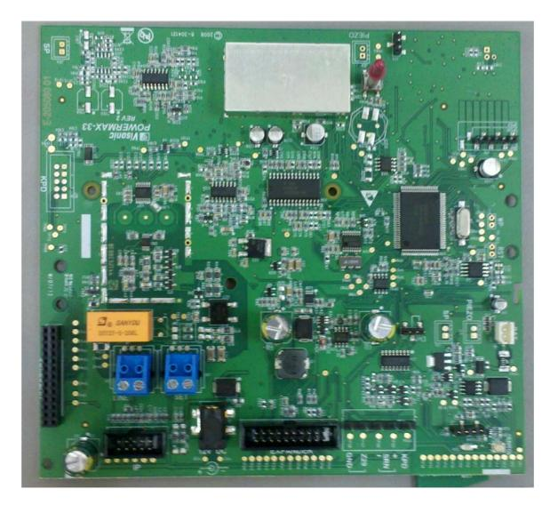
Photograph No.3 PMASTER-33 control panel motherboard
