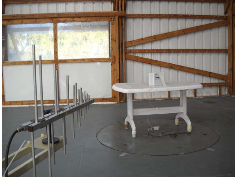
Photograph No.4 Setup for carrier and band edge spurious emission field strength measurements at the OATS in 30 – 1000 MHz range
