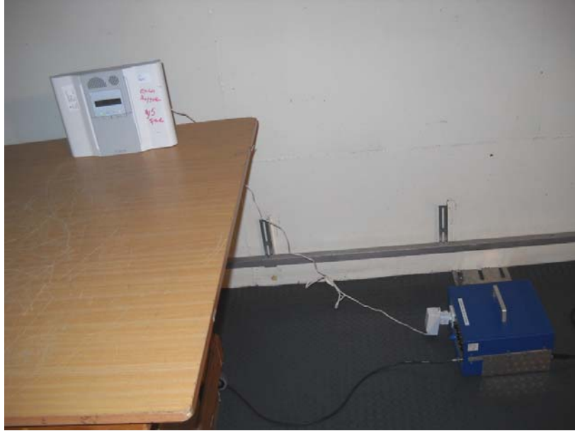
Photograph No.5 Setup for conducted emission measurements on AC power lines
