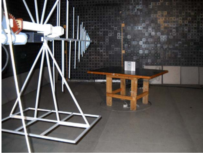
Photograph No.2 Setup for spurious emission field strength measurements in the anechoic chamber in 30 – 1000 MHz range
