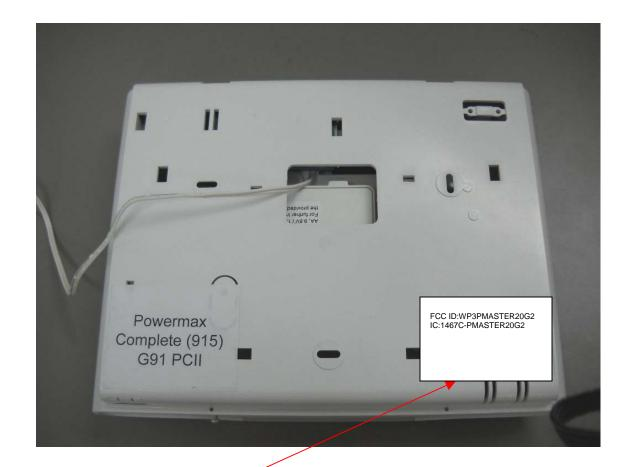
Label with FCC ID:WP3PMASTER20G2 and IC:1467C-PMASTER20G2 will be located at the rear side of the panel.
