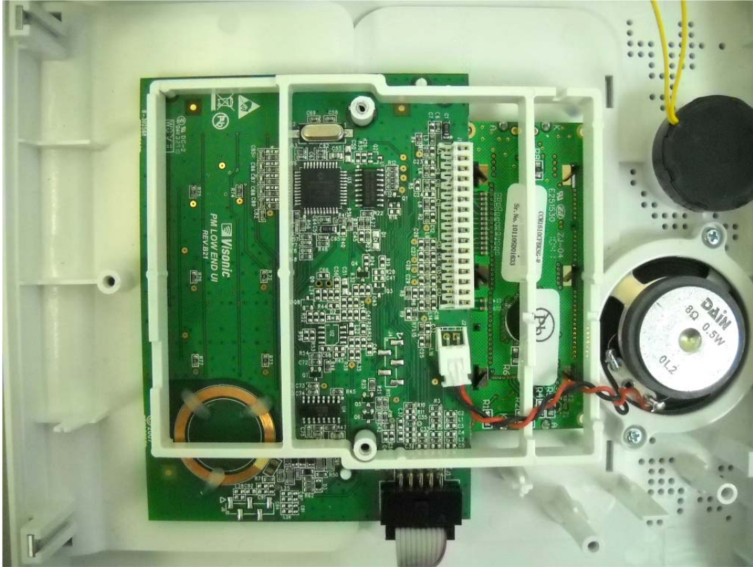
Photograph No.3 PMASTER-30 control panel internal view with motherboard removed Proximity module in the EUT case
