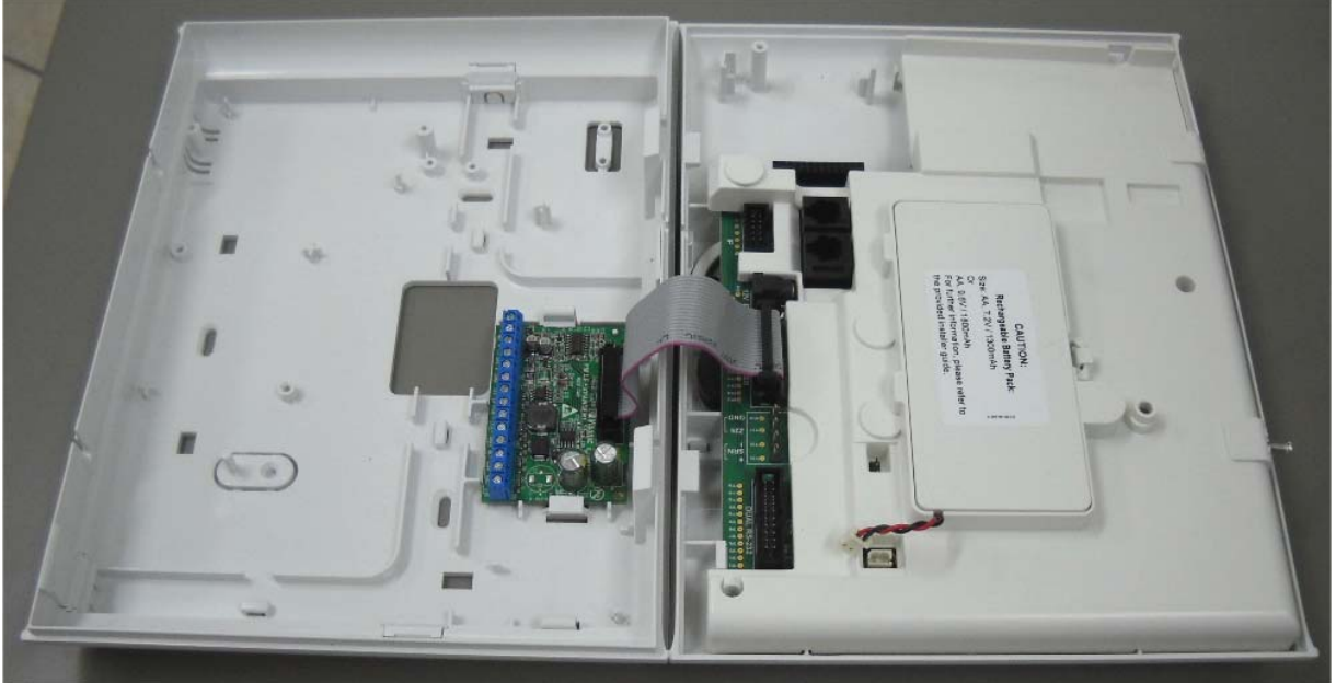
Photograph No.1 PMASTER-30 control panel internal view
