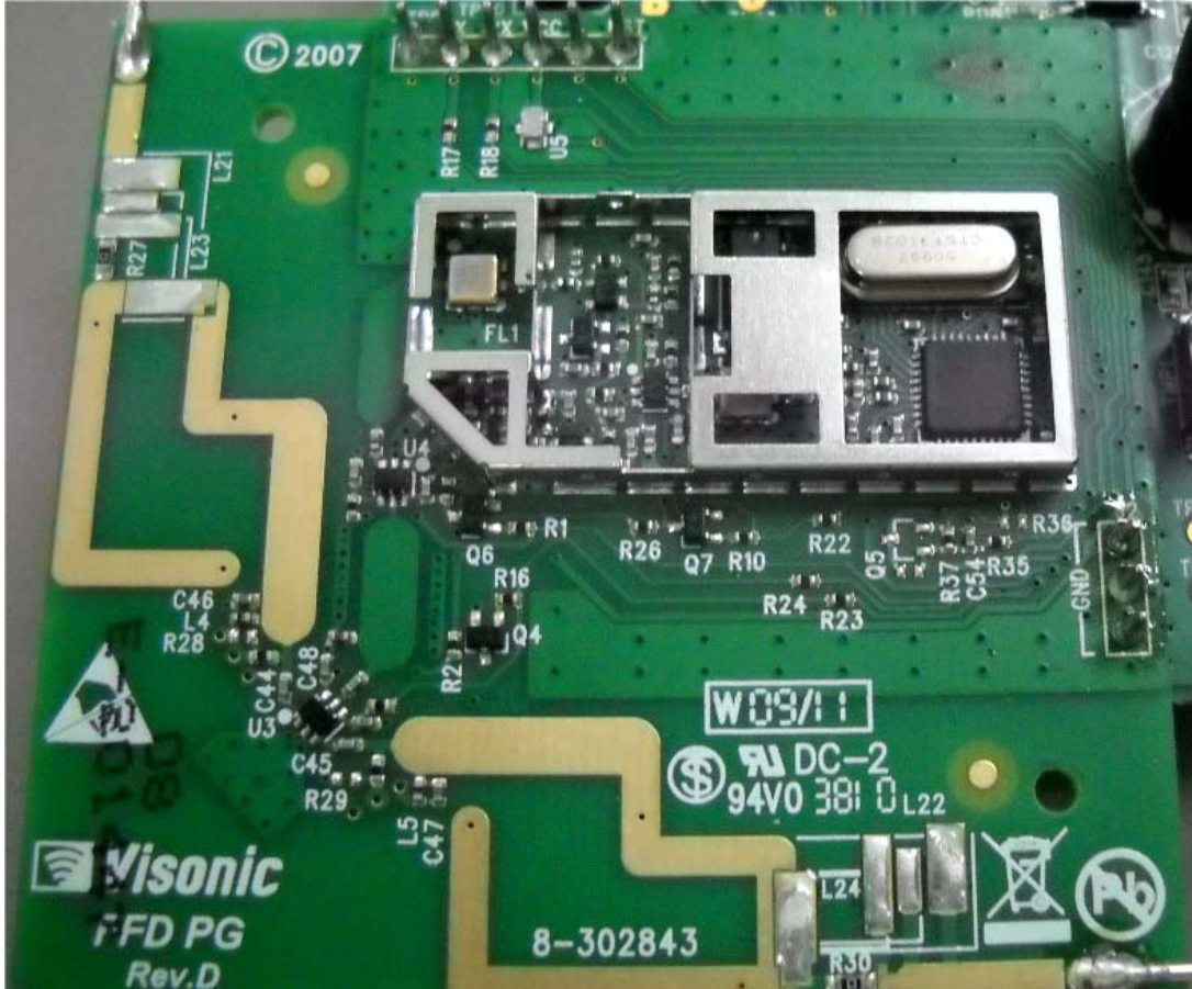
Photograph No.7 FFD RF module without shield
