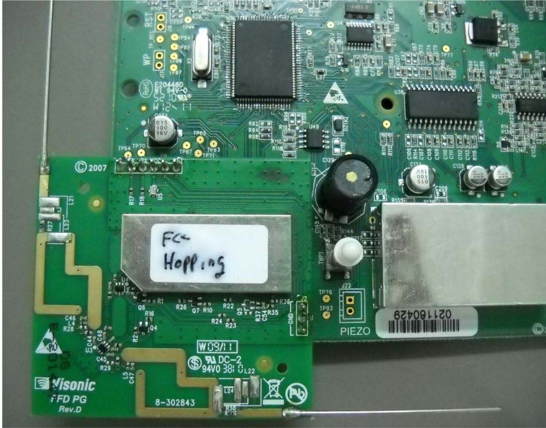
Photograph No.4 PMASTER-30 control panel motherboard with FFD module
