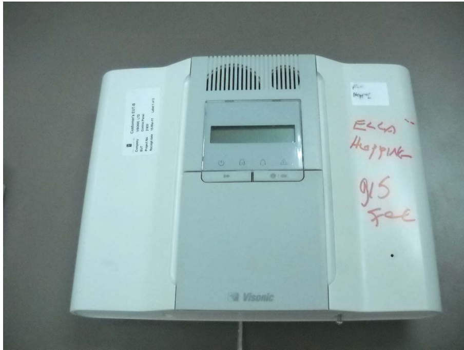
Photograph No.1 PMASTER-30 control panel front view
