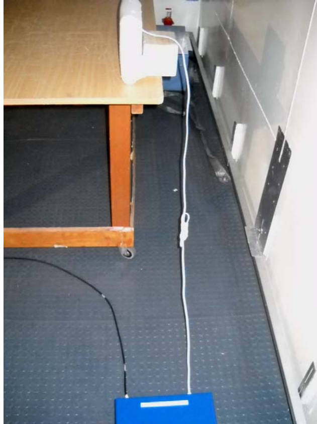
Photograph No.6 Setup for conducted emission measurements on AC power lines
