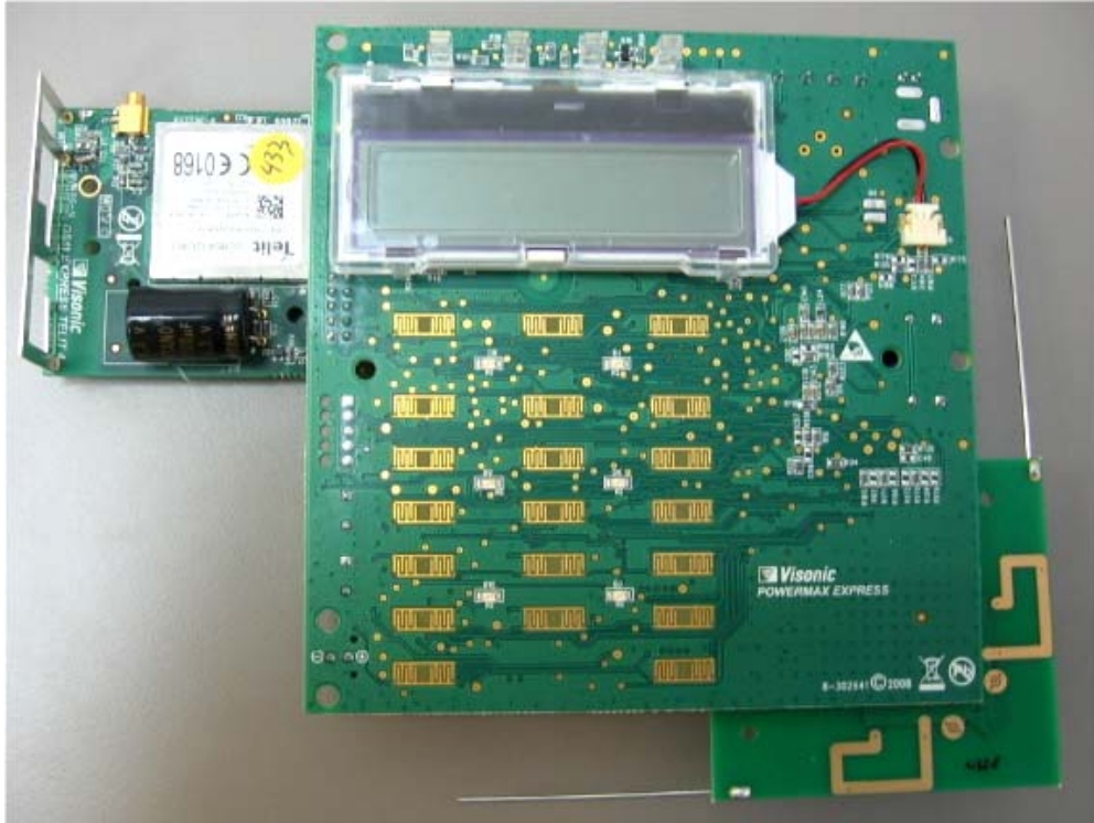
Photograph No.5 Control panel motherboard with 2 radio modules second side view
