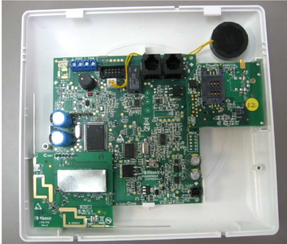
Photograph No.3 PowerMaster-10 G2 control panel internal view
