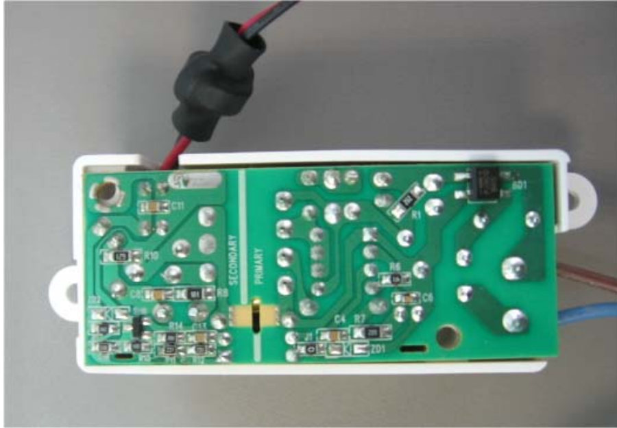
Photograph No.13 Power supply PCB view
