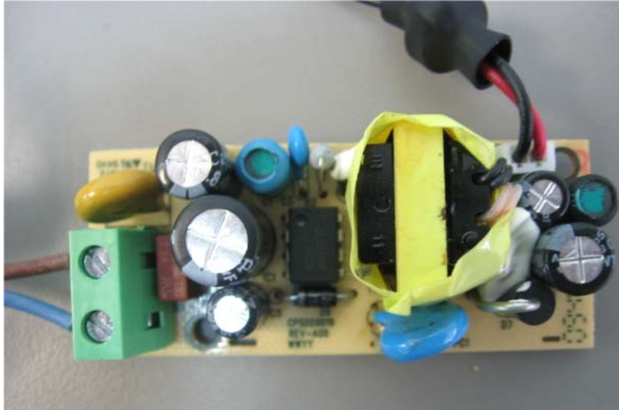
Photograph No.14 Power supply internal view
