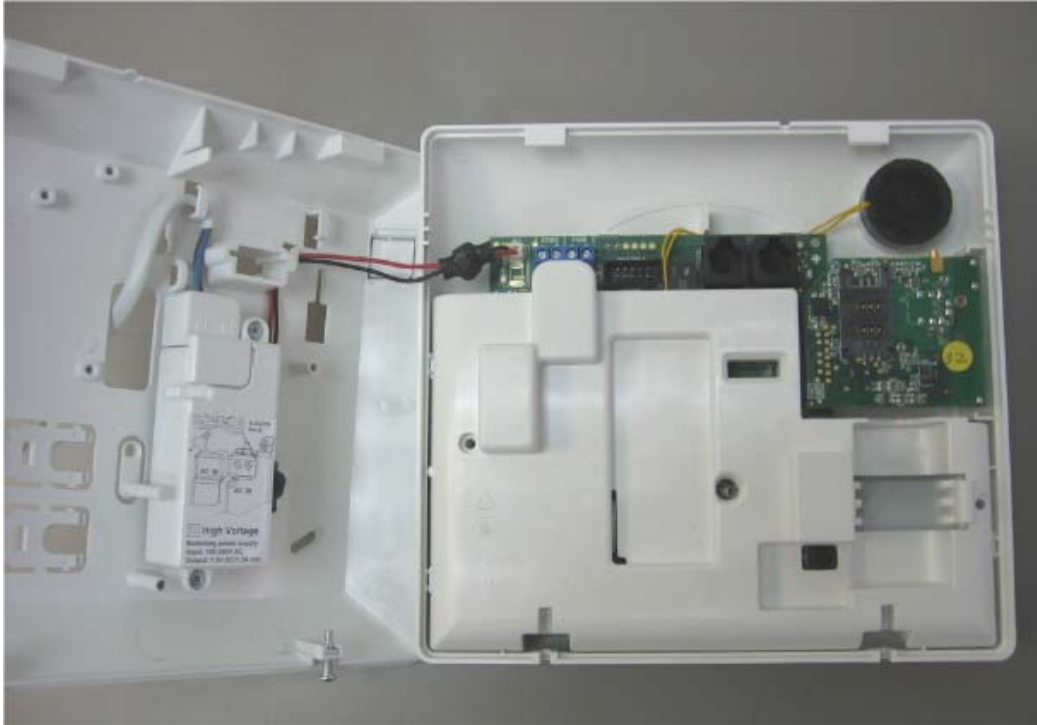
Photograph No.1 PowerMaster-10 G2 control panel internal view
