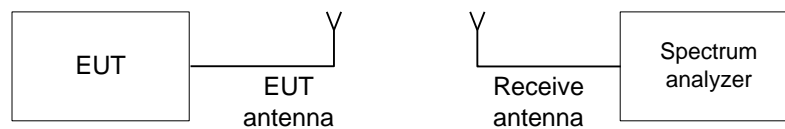
Figure 7.1.1 The 20 dB bandwidth test setup
