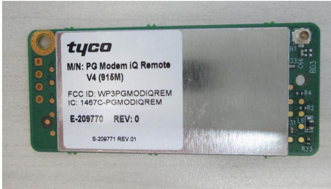
Photograph No.1 PG Modem iQ Remote Component side of the RF PCB
