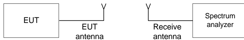
Figure 7.1.1 The 20 dB bandwidth test setup
