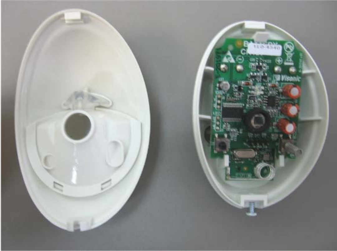
Photograph No.1 Digital PIR detector internal view
