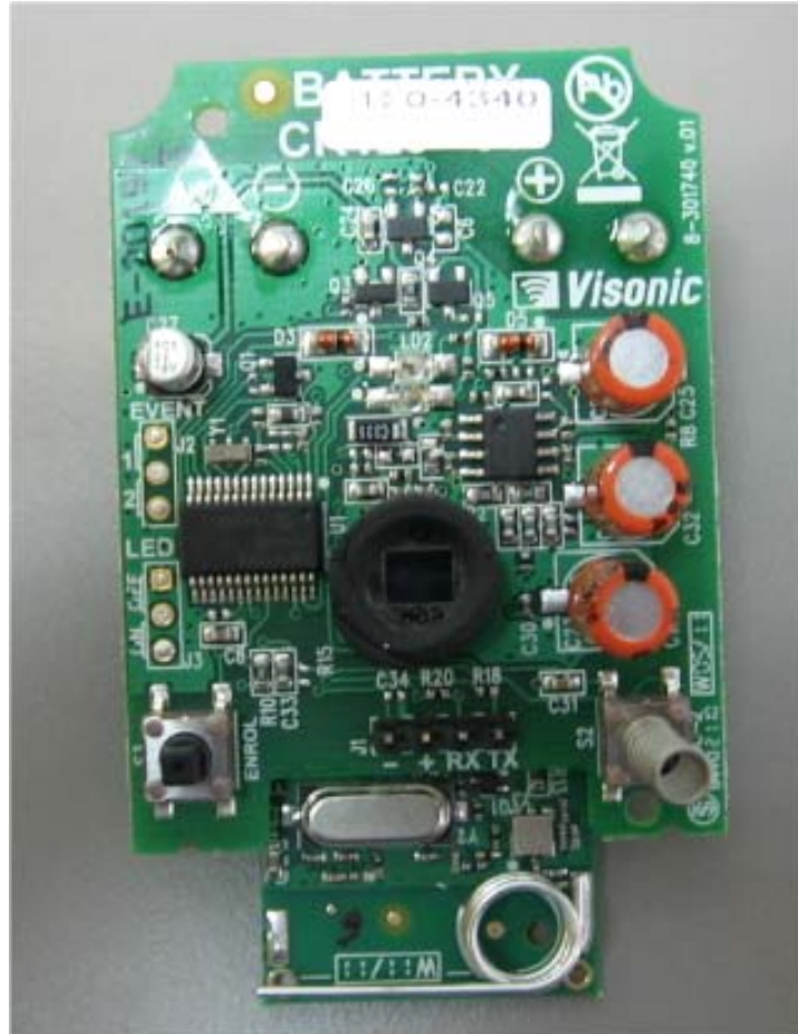
Photograph No.2 Digital PIR detector PCBs front view
