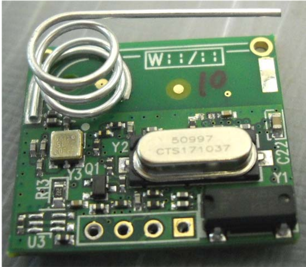
Photograph No.4 Detector RFD module front view
