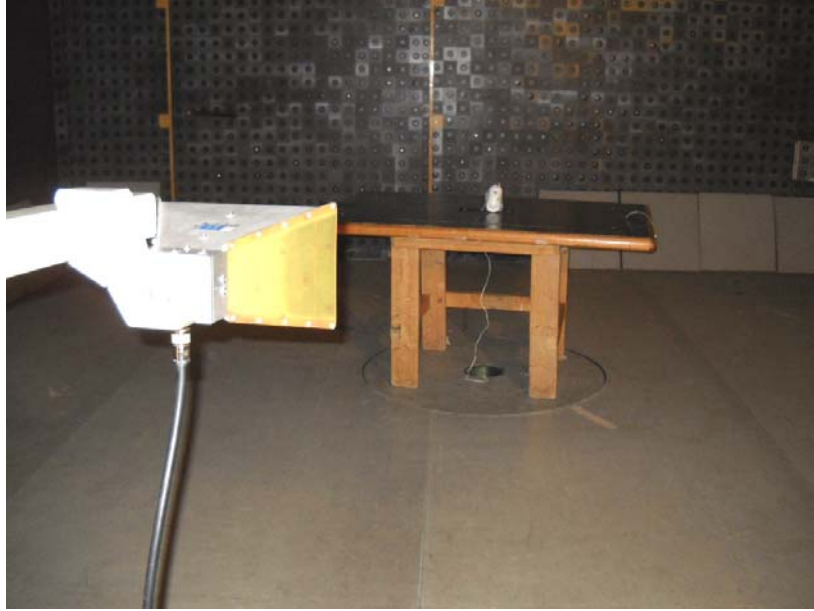
Photograph No.3 Setup for spurious emission field strength measurements in the anechoic chamber above 1000 MHz range
