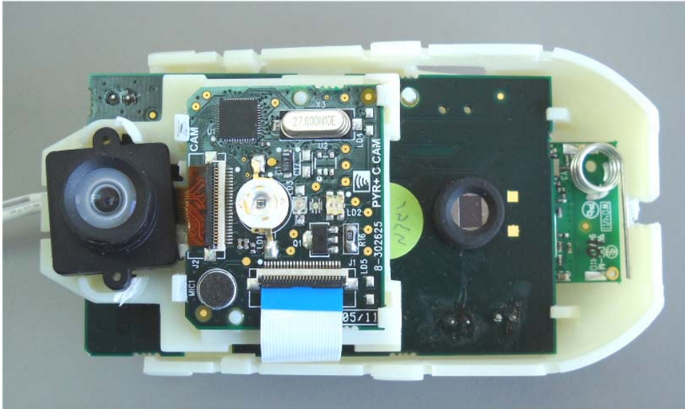
Photograph No.2 Digital PIR detector with camera internal view
