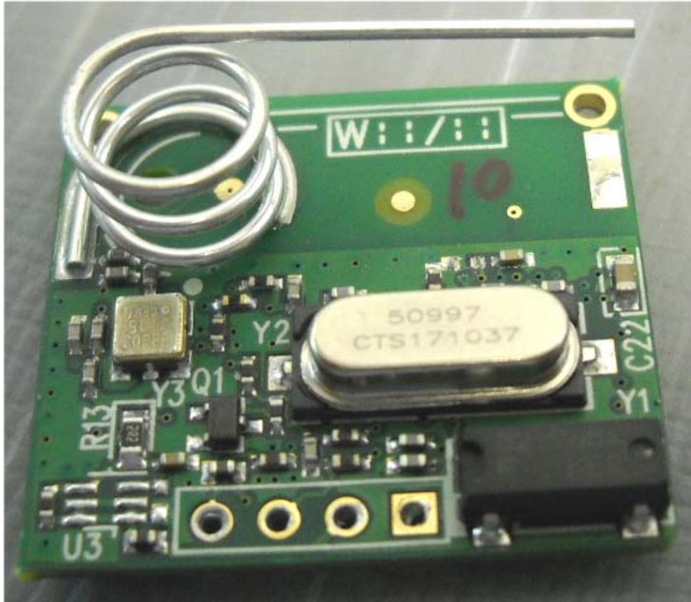
Photograph No.6 Detector RFD module front view
