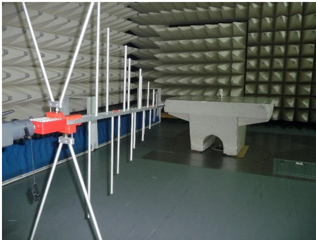
Photograph 8.1.1 Setup for final radiated emission measurements, general view
