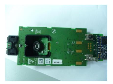
Photograph No.5 Outdoor PIR Detector Component side of the RF PCB (antenna assembly)
