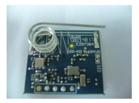
Photograph No.6 Outdoor PIR Detector Print side of the RF PCB
