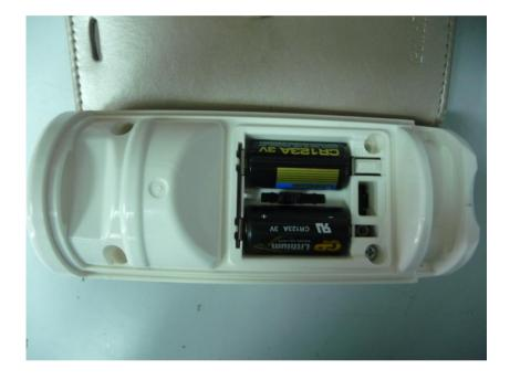
Photograph No.2 Outdoor PIR Detector Internal view (battery cradle removed)
