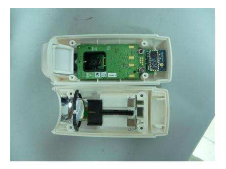
Photograph No.3 Outdoor PIR Detector Component side of the main PCB
