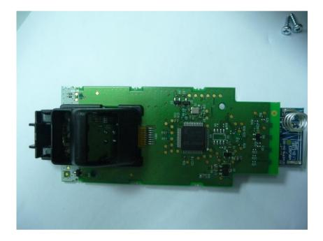
Photograph No.4 Outdoor PIR Detector Print side of the main PCB
