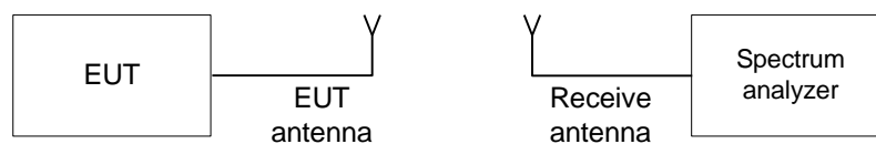
Figure 7.1.1 The 20 dB bandwidth test setup
