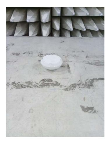
Photograph No.4 Setup for spurious emission field strength measurements, EUT close view
