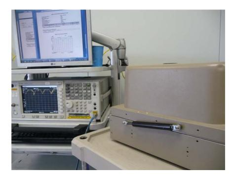
Photograph No.5 Setup for band edge emission and hopping parameters measurements
