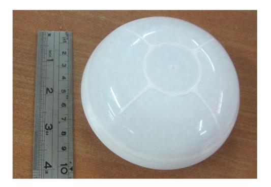
Photograph No.1 MP-862 PG2 PIR presence/security detector front view
