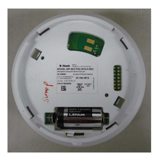
Photograph No.3 MP-862 PG2 PIR presence/security rear side view with backplane removed
