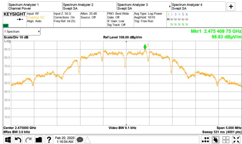
Plot 7.5.14 Peak spectral power density at mid frequency within 6 dB band ch.25, Antenna 2
